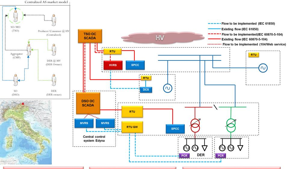
Aggregation of information in RT at TSO-DSO interconnection (HV/MV transformer)
