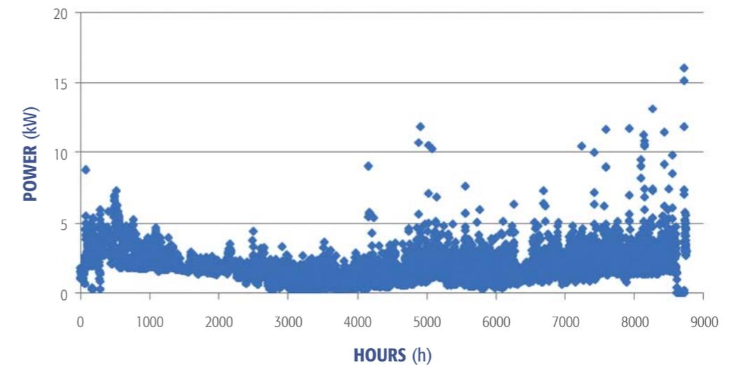
Figure 3. Main hourly powers of a Finnish electricity household customer over a one year period
